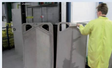
*Heat exchanger plate after chemical cleaning*
