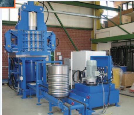
*Effective compaction of filter elements, Ignalina nuclear power plant (Lithuania)*
